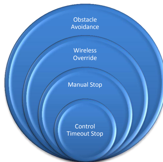
Figure 8 Layers of Protection
